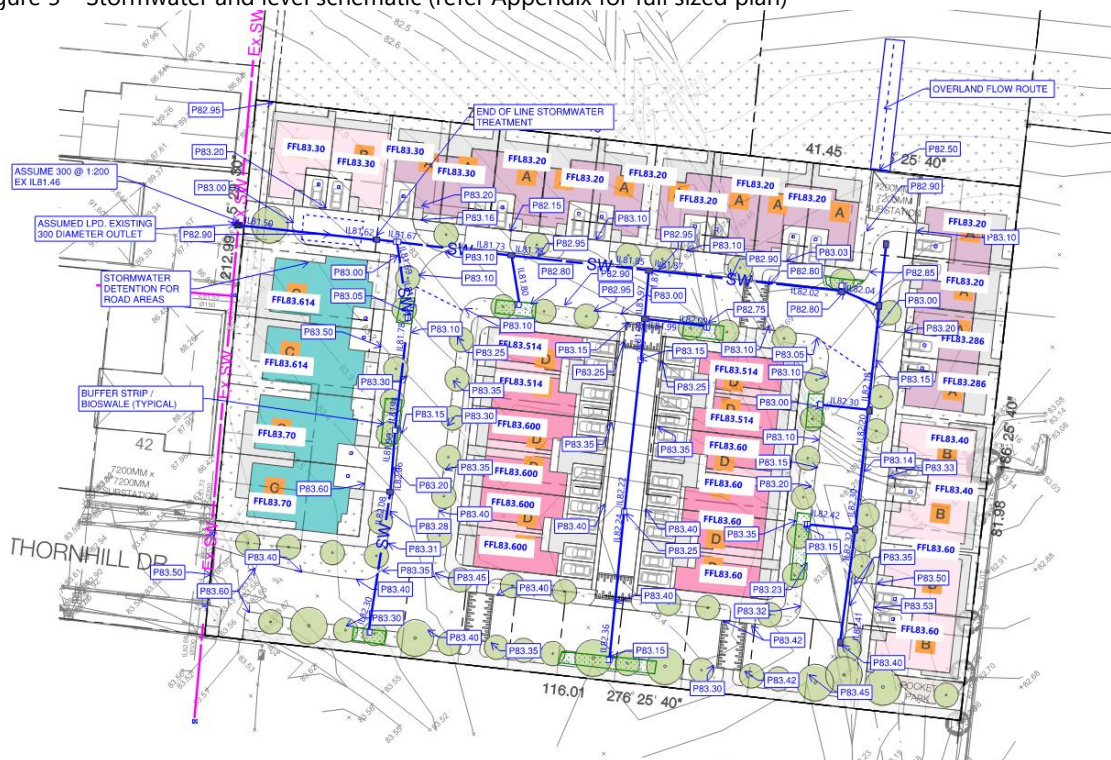
Figure 5 – Stormwater and level schematic (refer Appendix for full sized plan)
